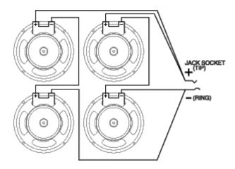
**Note:** Komet<sup>™</sup> Amplification recommends using a **16 Ohm** load with their amplifiers for the best sonic results.
