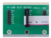
Eurorack connectors are usually orientated in a way that the -12V supply line is located at the bottom. The cmp1 module follows the same convention. The red line of the ribbon cable should show to the bottom of your bus board and at the bottom of your module. Refer to the figure above.
