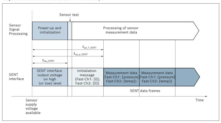
Values for the indicated times are available on request and are made available by Bosch Rexroth.
