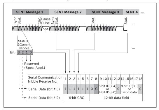
In the "slow-channel / slow-data", characteristic sensor data like coefficients, parameters, error information messages, OEM data, and so on are transmitted.
