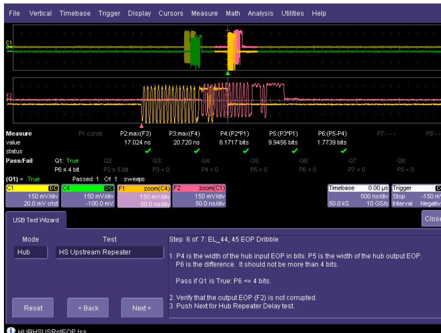
Figure 37. Hub upstream repeater end of packet dribble
