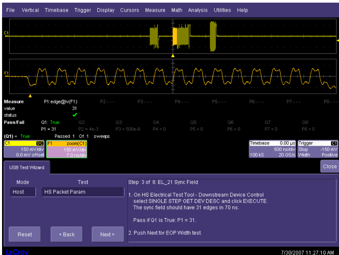
Figure 24. Host High-Speed packet parameters trace
