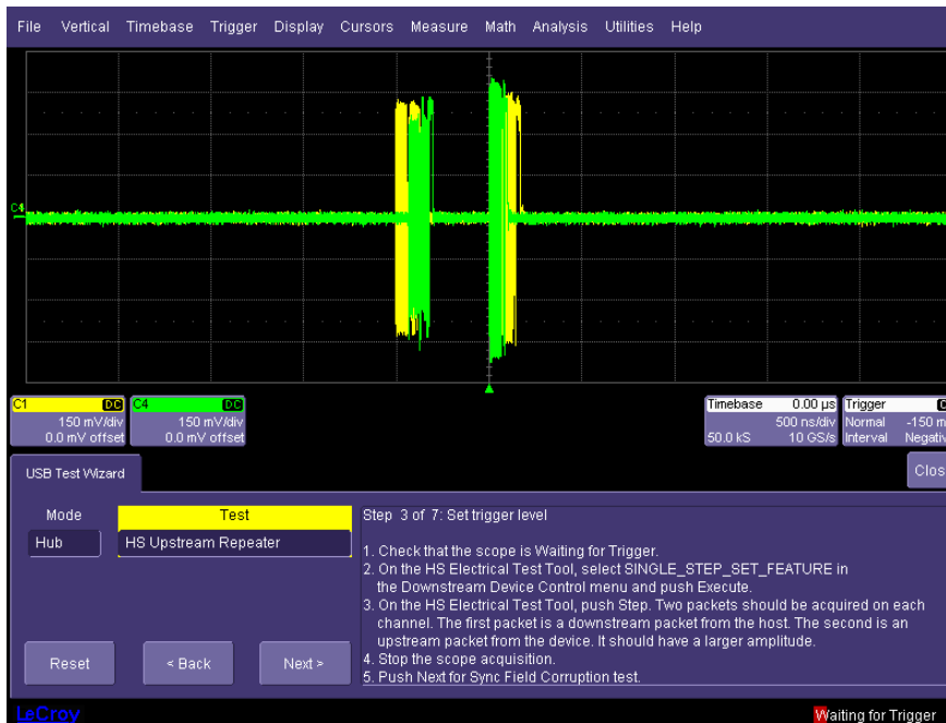
Figure 35. Initial signal acquisition for hub upstream repeater test
