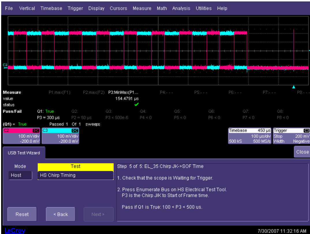
Figure 27. Chirp to Start of Frame Time
