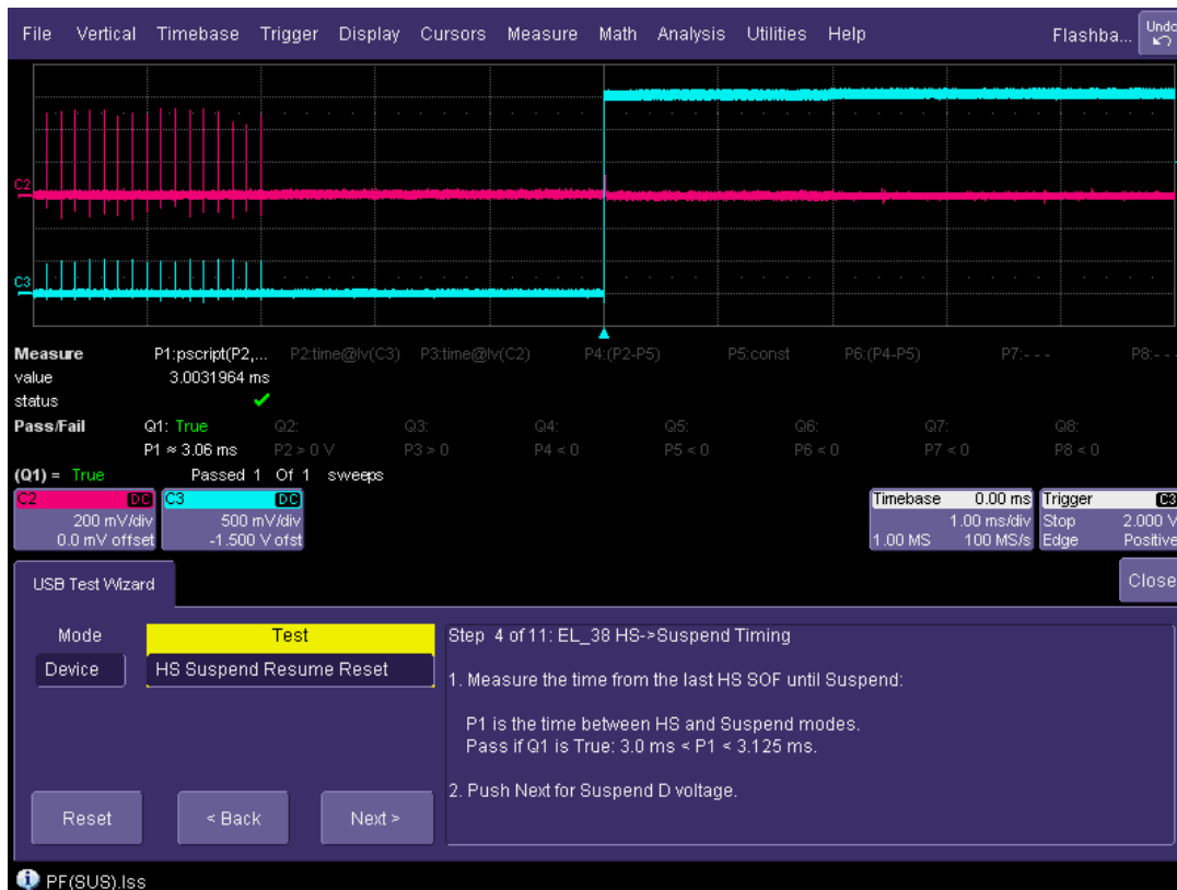
Figure 30. Time from Last Start of Frame to Device Suspend
