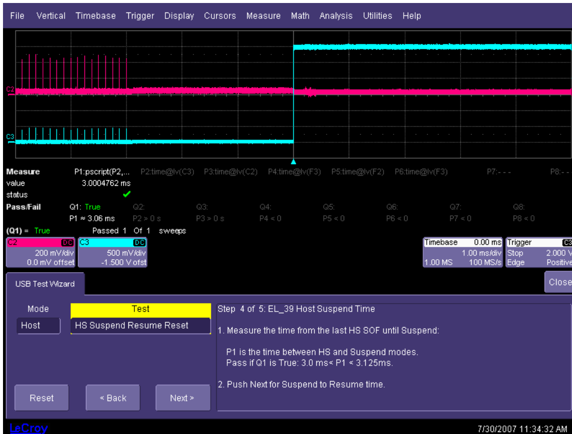
Figure 29. Time from Last Start of Frame to Host Suspend
