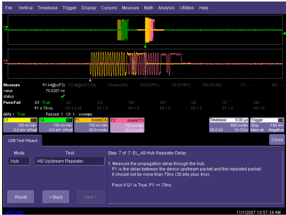
Figure 38. Hub upstream repeater delay
