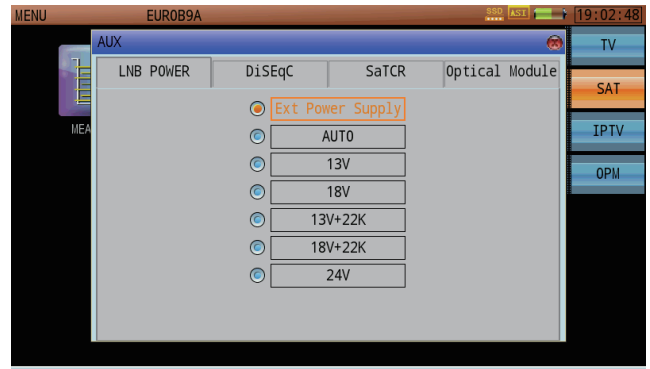
Figure-11 Remote Feeding and Control Signal Setting
