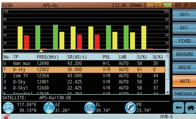
Figure-10 Display Max. 12 Transponders Signal Quality to Align Dish Antenna
