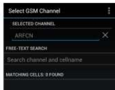
GSM cell lock: ARFCN selection. A loaded cell file can be searched for matching cells.
