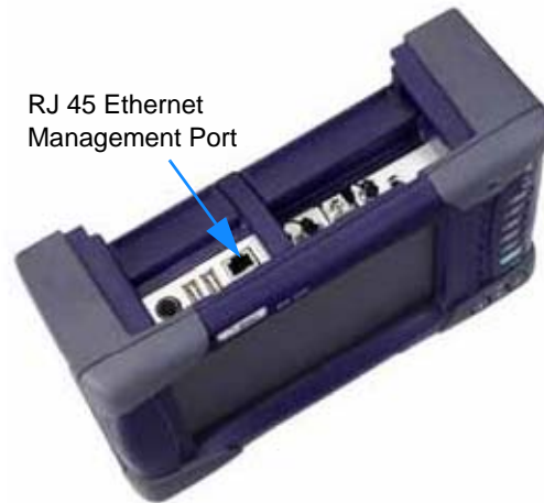
Figure 107 MTS/T-BERD 6000A Ethernet Management Port
