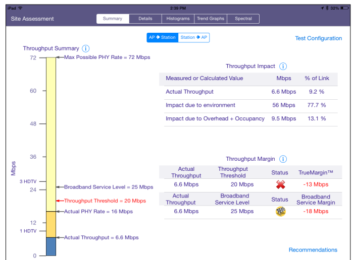
Site assessment analyze throughput and identifies slowdowns
