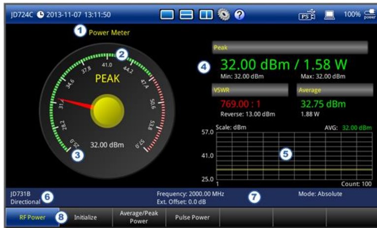
Figure 62 RF power measurement screen
