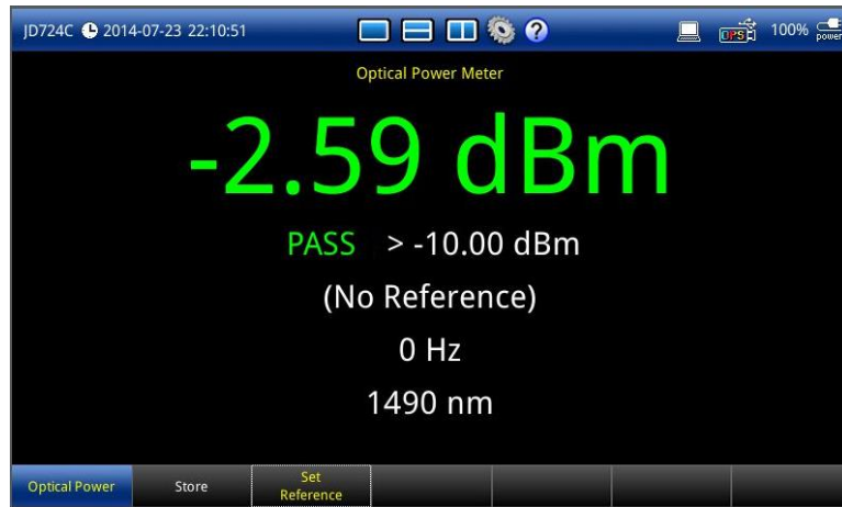
Figure 74 Absolute optical power measurement
