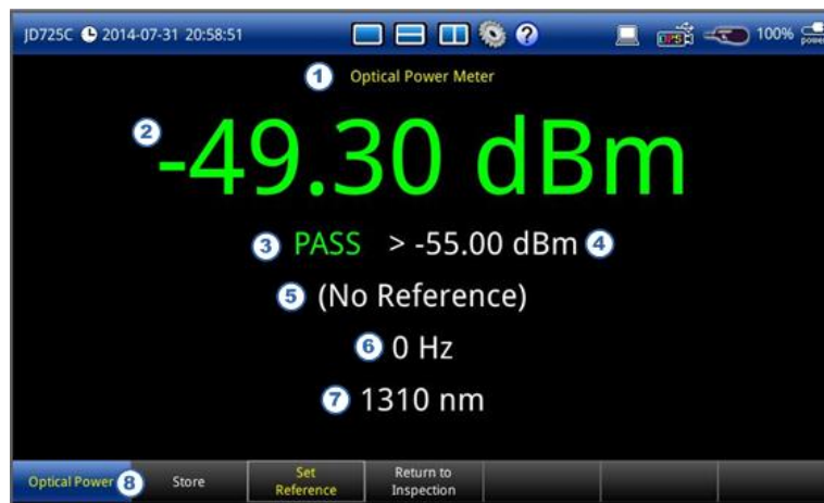
Figure 70 Optical power measurement screen
