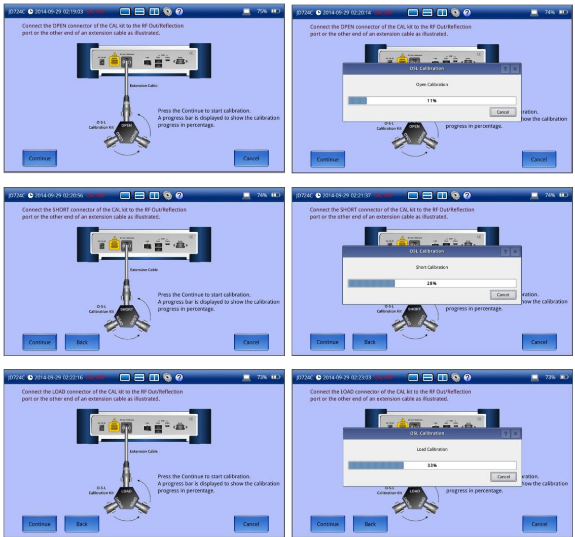
Figure 7 O-S-L calibration on JD724C using Y-Cal kit
