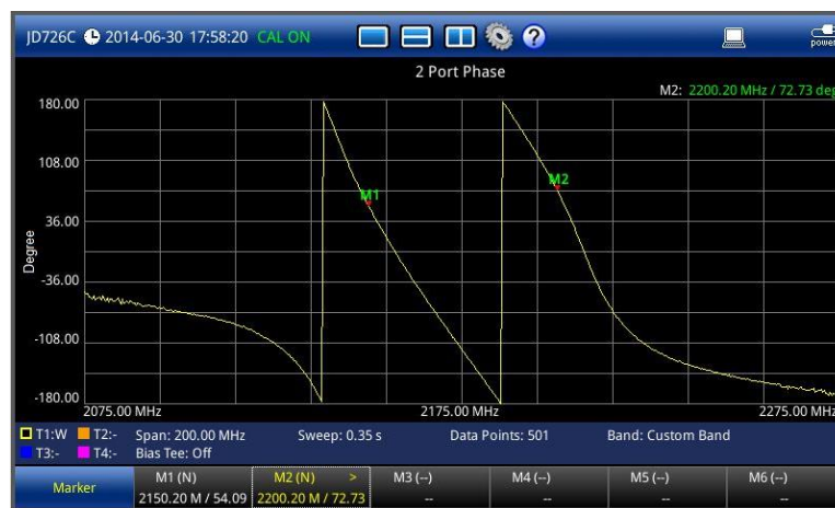
Figure 60 2 port phase measurement screen (single layout)
