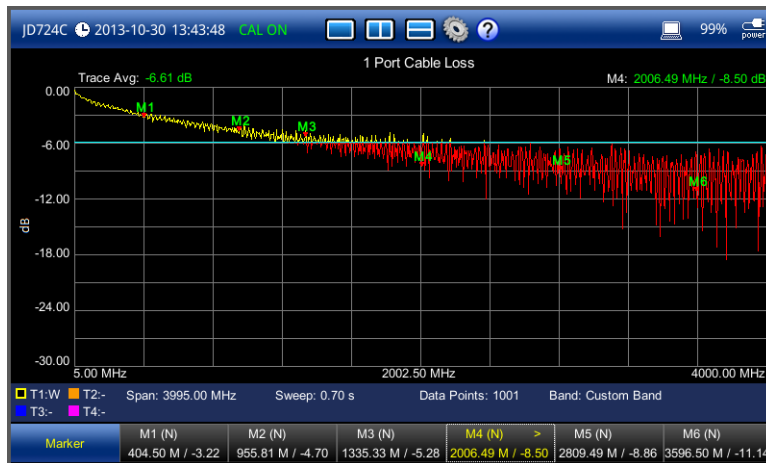
Figure 37 1 port cable loss measurement screen (single layout)
