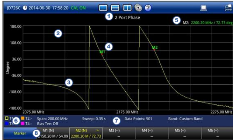
Figure 56 2 port phase measurement screen
