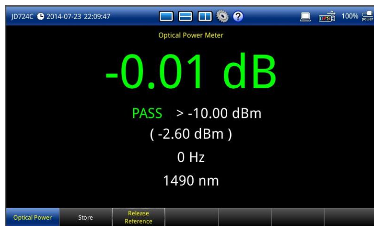
Figure 75 Relative optical power measurement vs. reference
