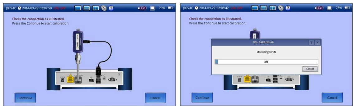
Figure 10 e-Calibration on JD724C using EZ-Cal kit
