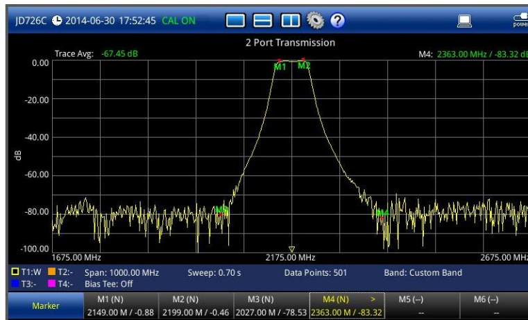
Figure 55 2 port transmission measurement screen (single layout)
