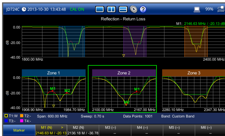
Figure 21 Reflection return loss measurement screen (zoom zones)
