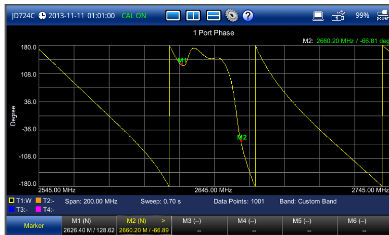
Figure 43 1 port phase measurement screen (single layout)
