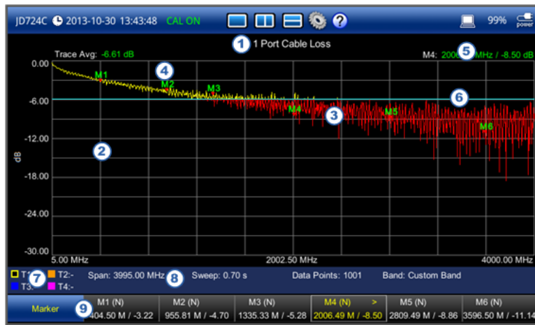
Figure 33 1 port cable loss measurement screen
