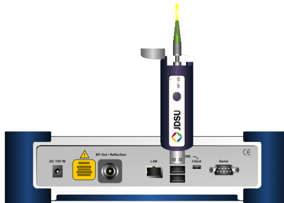
Figure 73 Cable connection diagram for optical power meter
