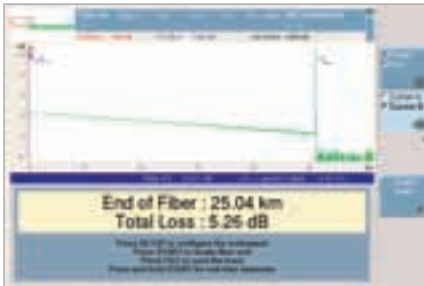
Figure 2 Fault locator mode
