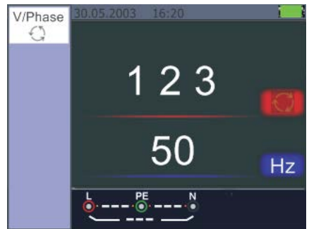
Figure 23 Phase Sequence screen-when connected in clockwise direction.
