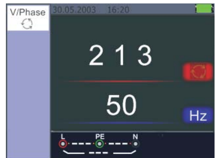
Figure 24 Phase Sequence-When connected in counter-clockwise manner
