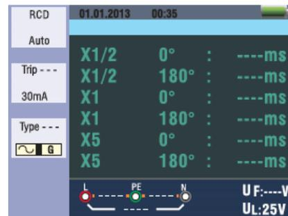
Figure 16 RCD Auto Function Screen
