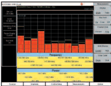
With Option 27, channel scanner measures power of multiple transmitters.
