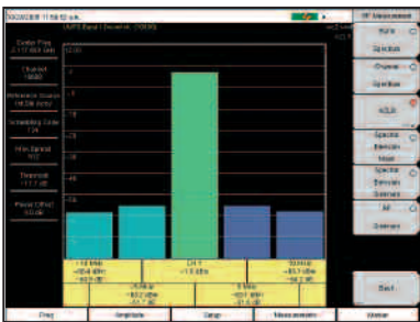
The ACLR screen shows the power levels for the main channel as well as two adjacent channels.
