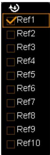
When the REF function is enabled, you can select different color for each reference waveform, set the source of each reference channel, adjust the vertical scale and position of the reference waveform and save the reference waveform to internal or external memory as well as recall it when needed. For details, please refer to the introductions below.
