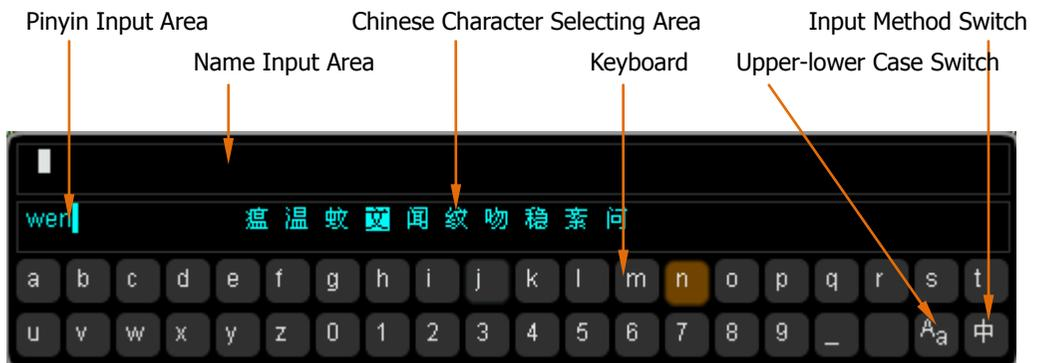
2. During the name input, you can press **Name** to select the “Name Input Area” and then press **Delete** to delete the Chinese characters on the left of the cursor one by one.
