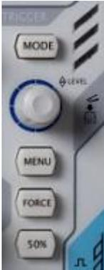
**MODE**: press this key to switch the trigger mode to **Auto**, **Normal** or **Single** and the state backlight of the current trigger mode would be illuminated.
