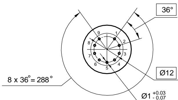
Electrode -to - lead connection diagram
