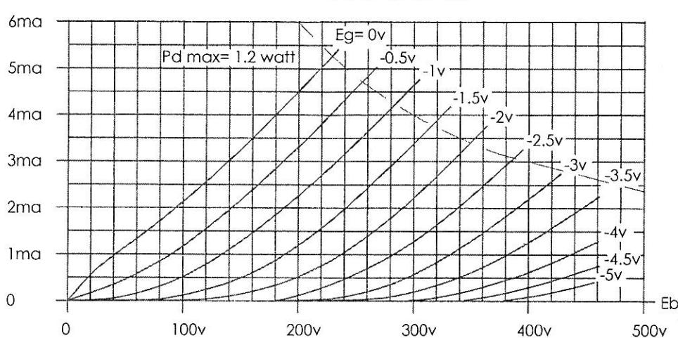
The 12AX7LP is a high mu dual triode with excellent linearity, making it a superior 12AX7 replacement.
