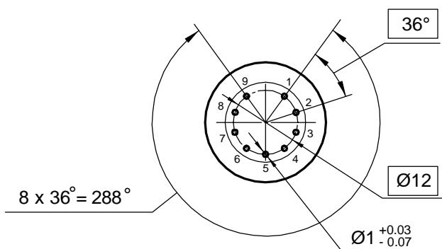
Electrode -to - lead connection diagram
