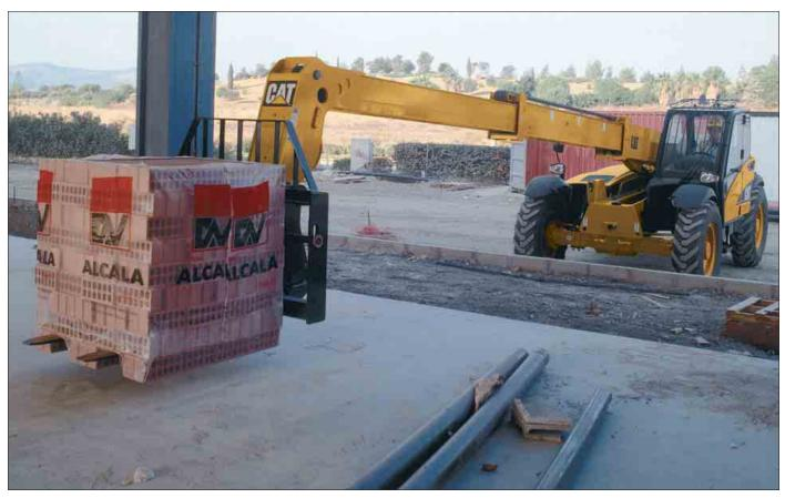
**Lift Height.** The TH350B can effectively and quickly place bricks, roofing materials and trusses to a maximum height of 11 000 mm.
