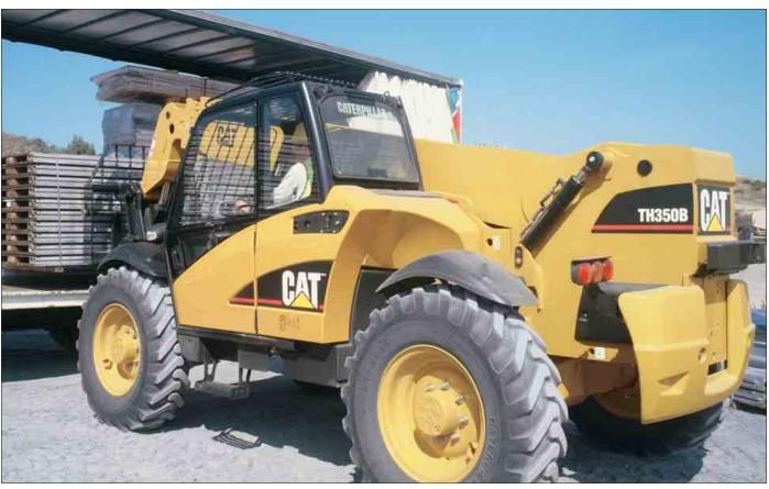
High Torque Rise Engine. The Cat 3054T engine, with its low emissions and high torque will give maximum performance whatever the conditions. For improved sound characteristics, a venturi tailpipe has been packaged inside the engine enclosure. The cooling system has been designed to work in the most challenging conditions.
