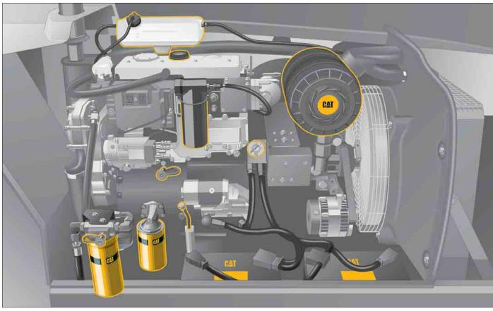
**Ease of Access.** Cost of ownership starts with ease of service. All Cat Telehandler service points are readily accessible and major components are easy to reach at ground level due to overall machine design.
