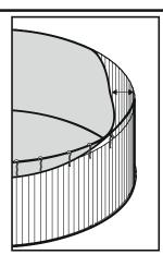
**NOTE:** The liner of the steel wall pool is designed to be smaller than the steel wall for technical reasons. If you find it difficult to assemble the liner, place the liner under the sun for one hour which will make it more pliable. You should then be able to assemble the liner step by step, stretching it by hand at the same time. This procedure will not damage the liner.
